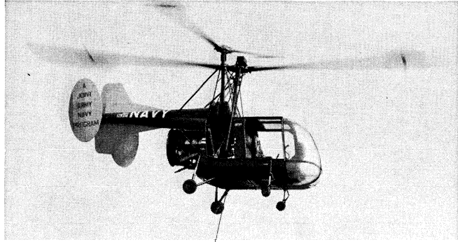
Kaman unmanned drone helicopter which may be operated either by means of a halter as shown, or remotely, by radio control
