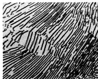
FIG. 6.—COARSE PEARLITE FORMED AT 1,300° F. (MAGNIFIED 2,000 X.)
