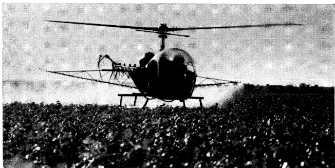
Bell helicopter equipped with spraying apparatus for agricultural use
