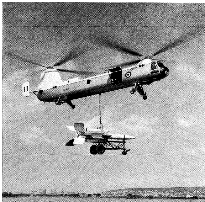
Bristol 192 (British) helicopter lifting a guided missile and its launcher
