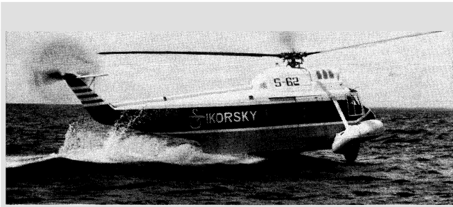
Sikorsky S-62, amphibious helicopter with flying-boat hull, landing on water
