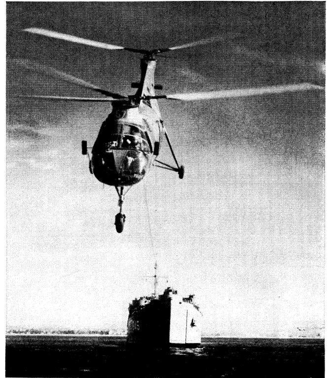
Vertol H-21 towing an LST at a forward speed of about 4 knots
