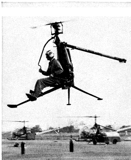
XROE-1 "Rotorcycle," a collapsible one-man helicopter manufactured by the Hiller Aircraft corporation
